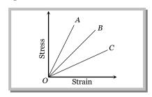
$Solution: \textbf{(c)} \quad \text{ From the graph } \tan\theta_C < \tan\theta_B < \tan\theta_A \ \Rightarrow \ Y_C < Y_B < Y_A \quad \therefore Y_{\text{Rubber}} \ < Y_{\text{Brass}} < Y_{\text{Steel}}$
